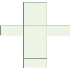
However, there is another way to consider the surface area of a prism. The top and bottom faces of a prism are the bases. The remaining faces are the lateral faces. Notice that if the lateral faces are opened out flat, they form one large rectangle. This rectangle is called the *lateral surface* of the prism.
