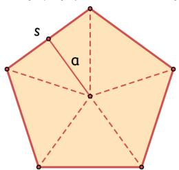
Notice the line drawn from the center of the figure to the midpoint of a side. This line is called an apothem. In any regular polygon, the center is the same distance from the midpoint of any side.
