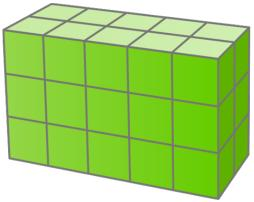
Note that the area of the base is the same as the volume of the first layer of the prism. This is the same as the number of 1 cm cubes in the bottom layer. The area of the base indicates the volume of one layer of the prism, while the height tells the number of layers.
